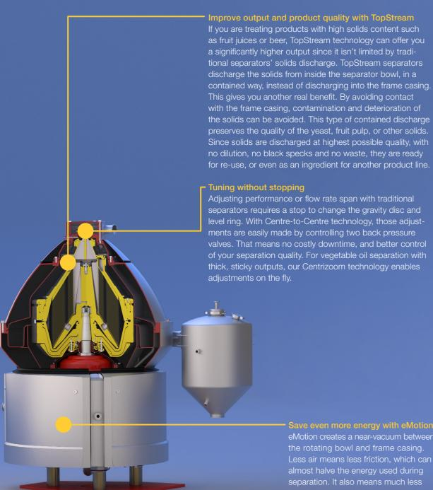
eMotion creates a near-vacuum between the rotating bowl and frame casing. Less air means less friction, which can almost halve the energy used during separation. It also means much less heat is generated. Hence you won't have to worry about buying and managing cooling solutions outside of the bowl, as you would with a traditional separator-with eMotion, frame temperatures will not exceed 30° Celsius.
