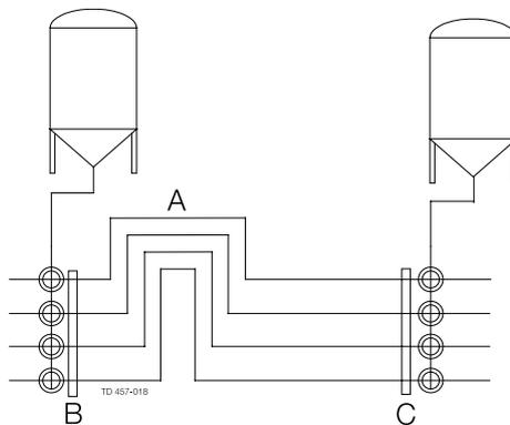
If space does not allow this, compensators can be inserted as shown below. For number and dimensions, please refer to supplier documentation.
