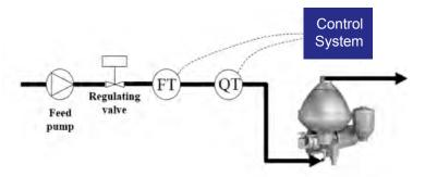
FT = Flow Transmitter QT = Turbidity Transmitter
