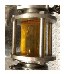
Polisher type: removes smaller particles > also reduces the chill haze
