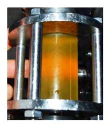
Clarifier type: removal of the bigger particles such as yeast or hop particles
