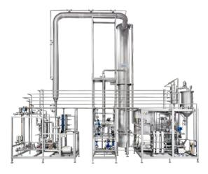
The Alfa Laval De-alc module provides a cost-effective and energy-efficient solution for removing alcohol from beer in a single pass. Its fully integrated system handles beer degassing, vacuum stripping, alcohol condensing, and culinary steam generation – ensuring premium taste with minimal energy consumption.
