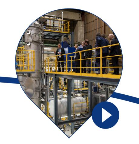
Alfa Laval Test & Training Centre The Alfa Laval Test & Training Centre is inaugurated in Aalborg, Denmark. A PureSOx test system at the facility is connected to a 2 MW MAN engine, allowing the scrubber to be pushed to its limits under controlled conditions. This accelerates the speed and quality of testing.
