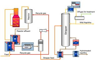
Fouling in the combined feed/effluent exchanger sometimes limits the throughput of the plant. It can even shorten the cycle-length, as heat exchangers need to be taken out for cleaning. Based on our experience in this service, Alfa Laval can recommend how to best operate and install heat exchangers that will maximize the uptime of your process – whether fouling is seen on feed side or on effluent side.
