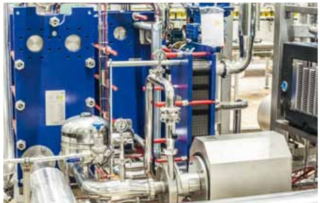
Soft drink mixer with Alfa Laval M10 and M6 heat exchangers and SolidC pump.
