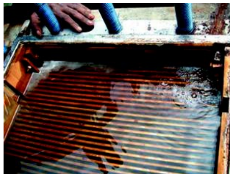
Fig. 9 Photo showing a leaking corner weld of a CPHE being air-bubble tested
